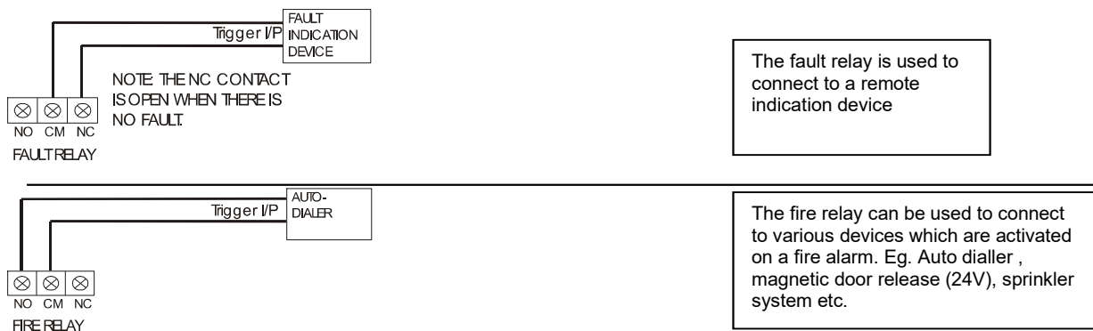
Typical auxiliary output wiring
