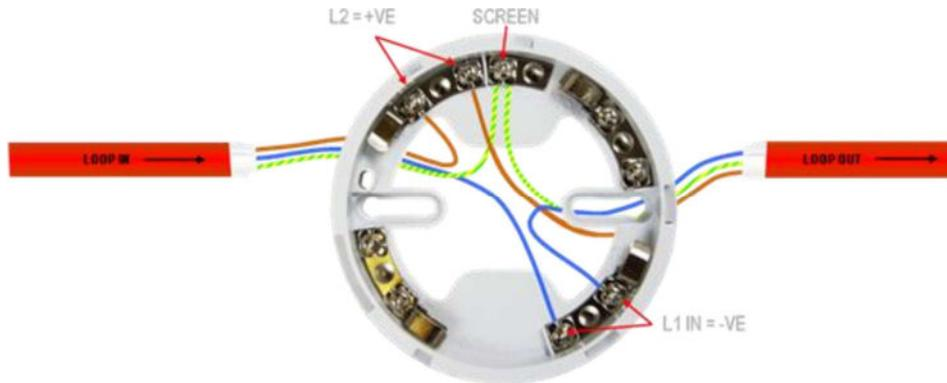
The connection for the detectors bases is made as follows:
