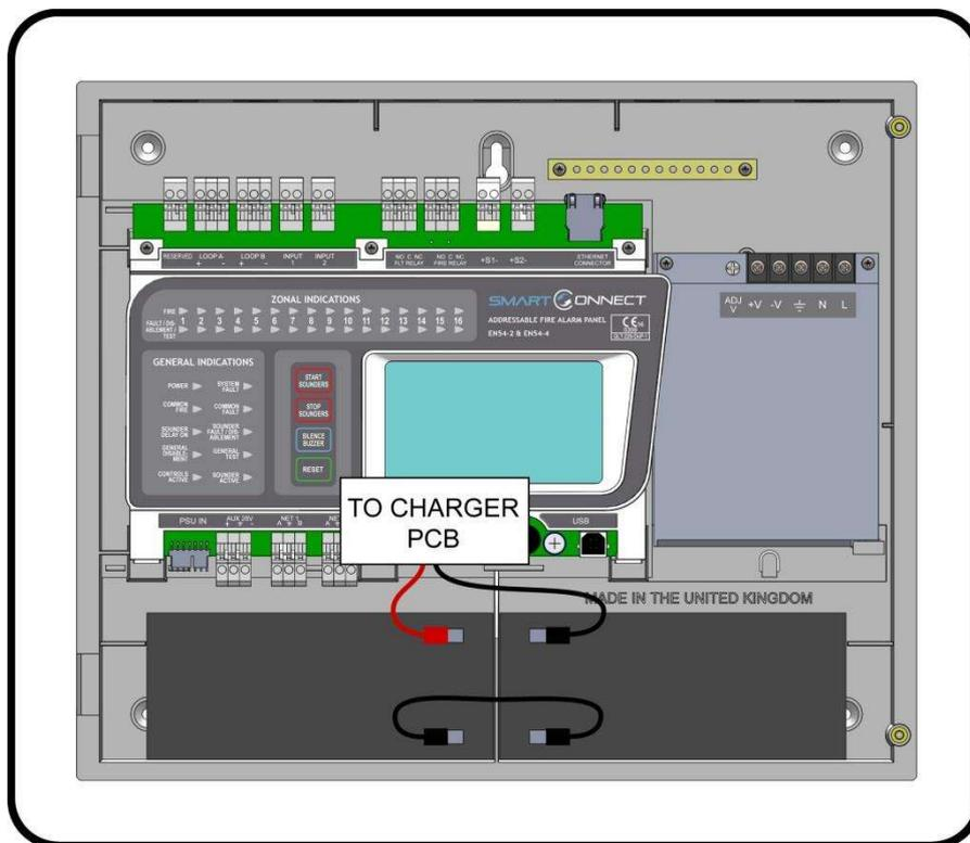
Figure 3: Battery location and connection details.
