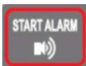
Press START ALARM to manually start the external sounders.
