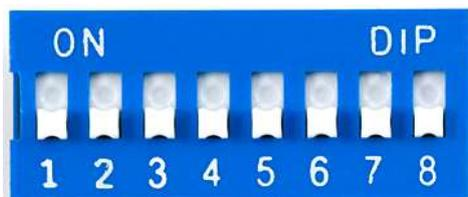
In general the **OFF** position represents binary 1, and the **ON** position represents binary 0, although certain devices may have this reversed (where OFF represents 0 and ON represents 1) so it is best to check the device documentation for further information.
