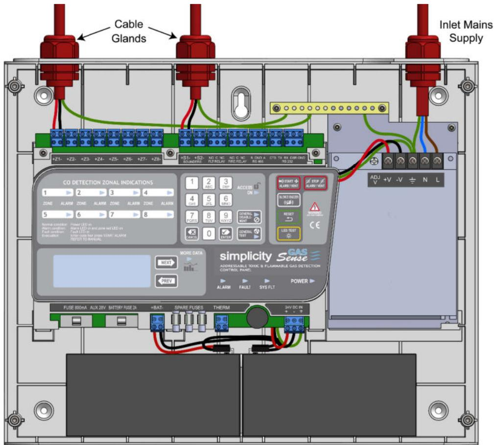
The 230V a.c. Mains cable must be fed into the enclosure via one of the cable entries at the top right corner of the back box. (Refer to "Connecting the Mains" on Following Page).
