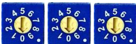
The address leads from left-to-right as hundreds, tens and units. For example if the first switch is set to 0, the second to 3 and the last to 5 the address will be set to 035.
