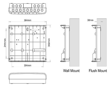
Fix the enclosure to the wall using the three mounting holes provided.
