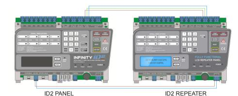
ID2 Repeater **ID2** Panel Description AUX 28V + 24V DC IN + Power for repeater AUX 28V -24V DC IN -Power for repeater RS485 B RS485 B Data connection **RS485 A RS485 A** Data connection RS485 GND RS485 GND Data connection screen
