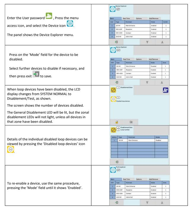
Once a loop device is disabled, the panel ignores any alarm or fault generated by the device. If all devices in a zone are disabled, the panel will indicate a zone disablement. If subsequently one or more devices in that zone are reenabled then the zone disablement indication will be automatically cancelled.
