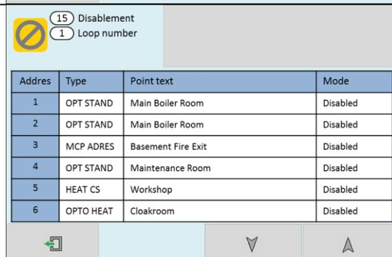
To re-enable a zone, use the same procedure, pressing the 'Enabled' selection circle.
