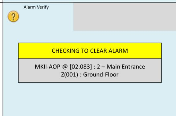
If the detector is still in the alarm state, the panel will enter the ALARM condition.
