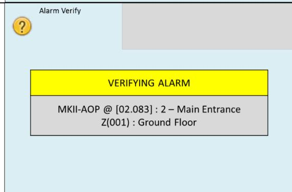
When the detector is in the confirmation phase, the detector alarm LED's will turn off and the panel will begin processing if the same detector is still in an alarm state for the selected time duration.
