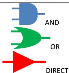
An AND / OR cause will request more inputs before activating the output.
