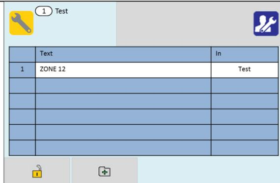
As devices are tested, the screen changes to show the recent tests. Use the arrow to scroll to view older tests if required.
