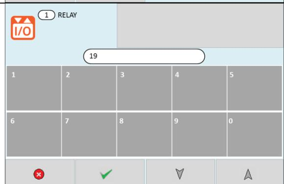
You can change the mode of each output to Programmable, Alarm, Fault or Tech. alarm.
