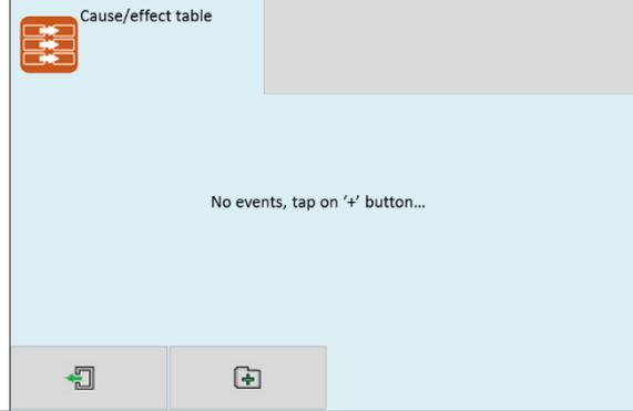
The panel displays the 'select cause' screen, Choose the cause type (Point, Local I/O, Zone or Panel). Depending on the input type chosen, the panel will display a list of sub options. For a 'Point' cause the options are:-
