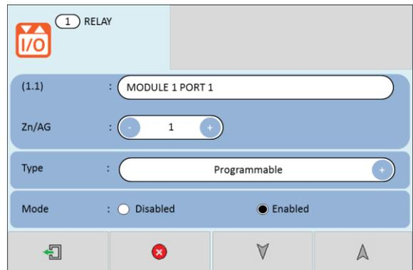
To change the text label of a module output, press on the text label field. This will display the panel keyboard. Enter the required text name, and then press the green tick to confirm.
