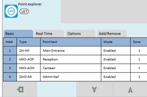
Once a loop device is disabled, the panel ignores any alarm or fault generated by the device. If all devices in a zone are disabled, the panel will indicate a zone disablement. If subsequently one or more devices in that zone are re-enabled then the zone disablement indication will be automatically cancelled.
