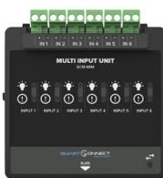
The SCM-MIM has six class B inputs that are commonly used to monitor and raise alarms from any specific ancillary equipment. Each Input is monitored for open or short circuits and can also be programmed to give a supervisory or alarm signal when active.
