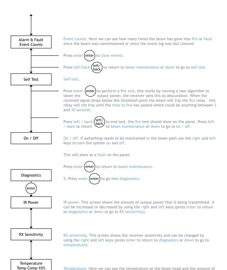
Temperature. Here we can see the temperature at the beam head and the amount of compensation being made for temperature (no adjustments can be made here).
