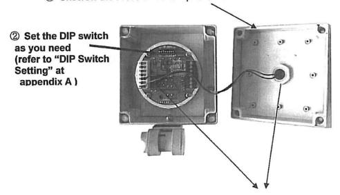
3 Let the applicable wires go through the cable gland of Back Cover and connect them to the terminal blocks
