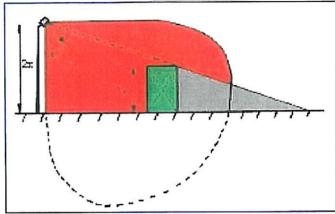
As a rule of thumb the detector is mounted twice as high as the highest object in the protected area.
