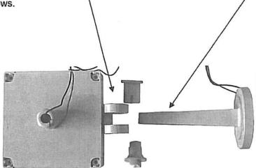
(5) Adjust the tilting angles of completed detector for your application situation/purpose.
