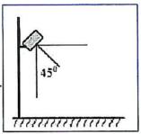
friendly fires. By pointing the detector down in an angle of 45° it allows you to fully utilize the Field of View. In this case one side of the Cone of Vision will cover the area horizontally and the other side of the Cone of Vision will cover the area vertically.
