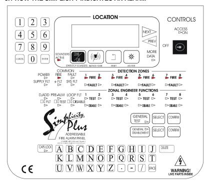
When the Simplicity Fire Alarm Panel is set into alarm by a Detector or Manual Call Point located in a zone that is not already in alarm it will: -
