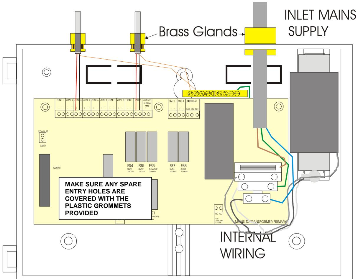
Figure 6: Detector and Sounder Circuit Connection
