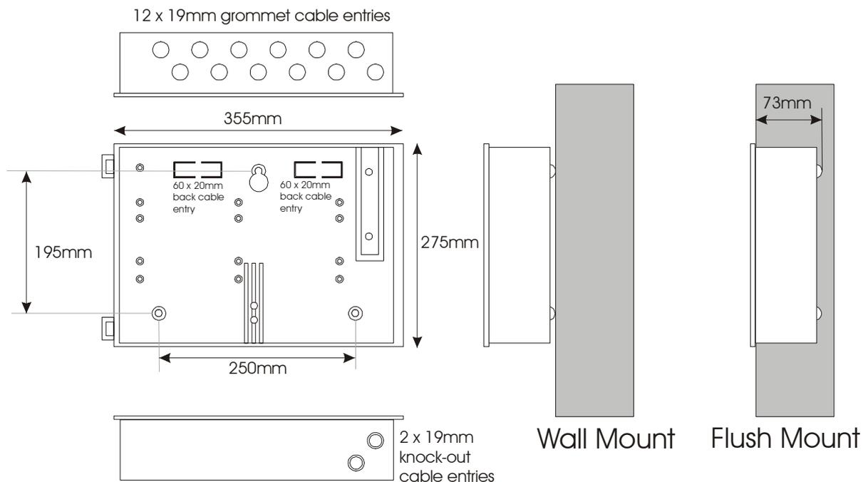
Fix the enclosure to the wall using the three mounting holes provided.
