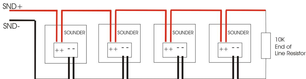
Note: If non-polarised alarm devices (eg some types of old mechanical bell, or a relay) are used, then a diode will have to be placed in line with the device to enable fault monitoring. They may also need a back EMF protection diode. (symptoms: Chattering sounder relays that don't turn off).
