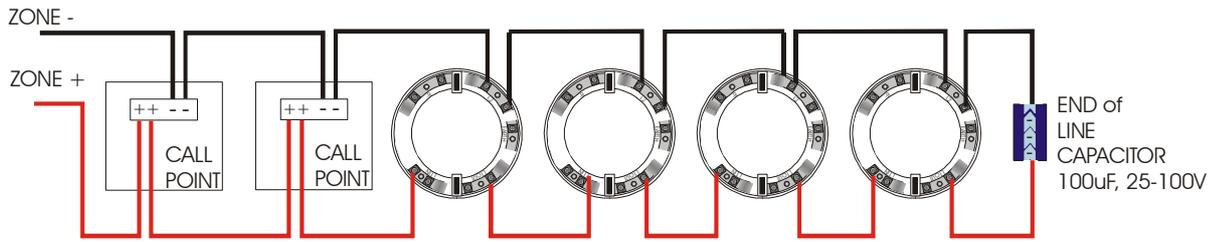
If ALL the call points are connected to the start of the zone, then conventional bases can be used instead of diode bases.
