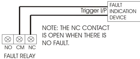
The fault relay is used to connect to a remote indication device
