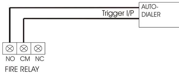
The fire relay can be used to connect to various devices which are activated on a fire alarm. Eg. Auto dialer , magnetic door release (24V), sprinkler system etc.
