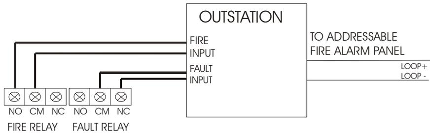
Here the relays are used to communicate with a larger addressable fire alarm system. An example use of this might be a warehouse, which uses several flame detectors, and needs to be part of a larger system.
