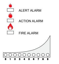
BARGRAPH of SMOKE LEVEL or AIRFLOW SPEED
