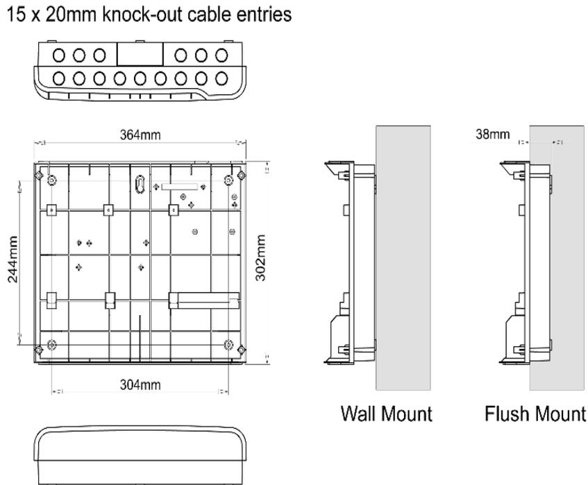
Fix the enclosure to the wall using the three mounting holes provided.
