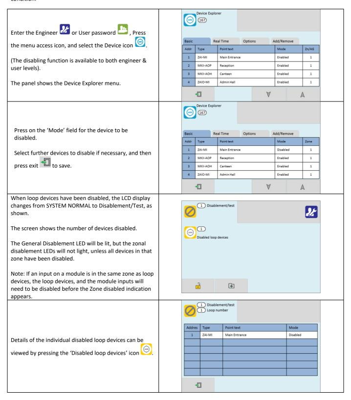
To re-enable a device, use the same procedure, pressing the 'Mode' field until it shows 'Enabled'.
