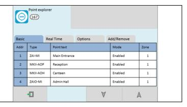
Once a loop device is disabled, the panel ignores any alarm or fault generated by the device. If all devices in a zone are disabled, the panel will indicate a zone disablement. If subsequently one or more devices in that zone are re-enabled then the zone disablement indication will be automatically cancelled.
