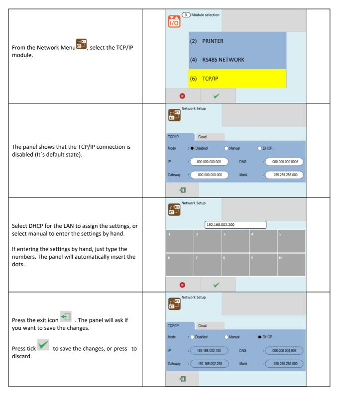
With only the TCP/IP configured, the panel will sit on a network, but would need 3rd party software on a PC to do anything useful. The cloud settings will need to be configured in order for the panel to link to the remote server.
