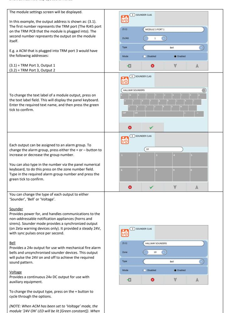
it is set to Bell, the 24V on LED will be flashing.
