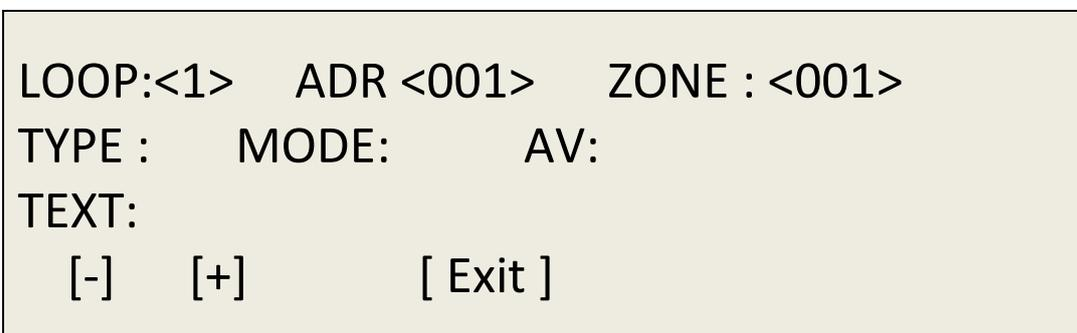
With left and right arrow keys you can select the address field of the loop or loop point selected. By pressing <+> <-> or up and down arrow keys you can increase or decrease these fields and move from one element to another.
