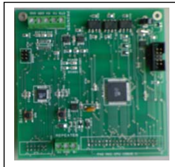
New CPU – 2 small surface mount ICs
