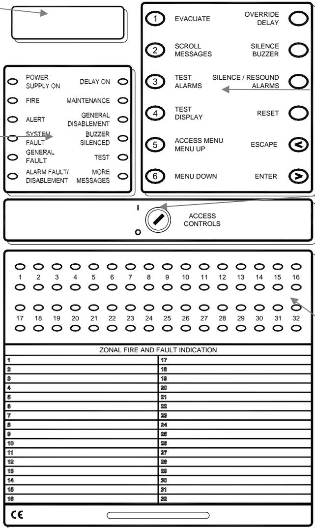
User controls. Only override delay is available without operating the access controls keyswitch
