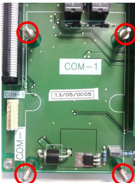
At the bottom of the PCB, just left of the LOOP 1 slot, will be where the QT/NC is to be fitted. There will be 4 spacers that the Network card will sit upon.
