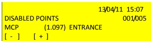
Alternatively, up to 10 disabled points (without indicating device type or address) can be displayed on one screen as follows.
