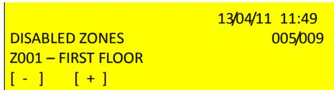
Alternatively, up to 10 disabled zones (without text labels) can be displayed in one screen as follows. Select any key followed by Level 1 password ( default 1111), and then Zones followed by Show Disabled Zone. Zones are displayed in groups of 10, with the symbol X underneath a zone which has been disabled. The next group of 10 zones can be displayed by pressing the + symbol. The - symbol can be used to go back 10 zones.
