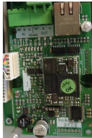
The Standard Network card provides an RS485 repeater connection, and an RS252 Printer connection.
