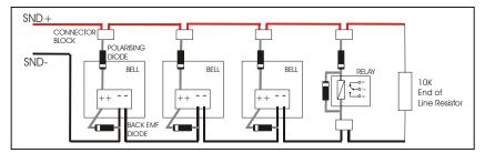
Note: If non-polarised alarm devices (eg some types of old mechanical bell, or a relay) are used, then a diode will have to be placed in line with the device to enable fault monitoring. They may also need a
