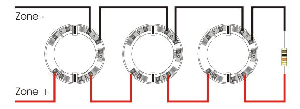
Call points should be connected to the start of the zone, so that removing a detector head will not remove power from the call points.
