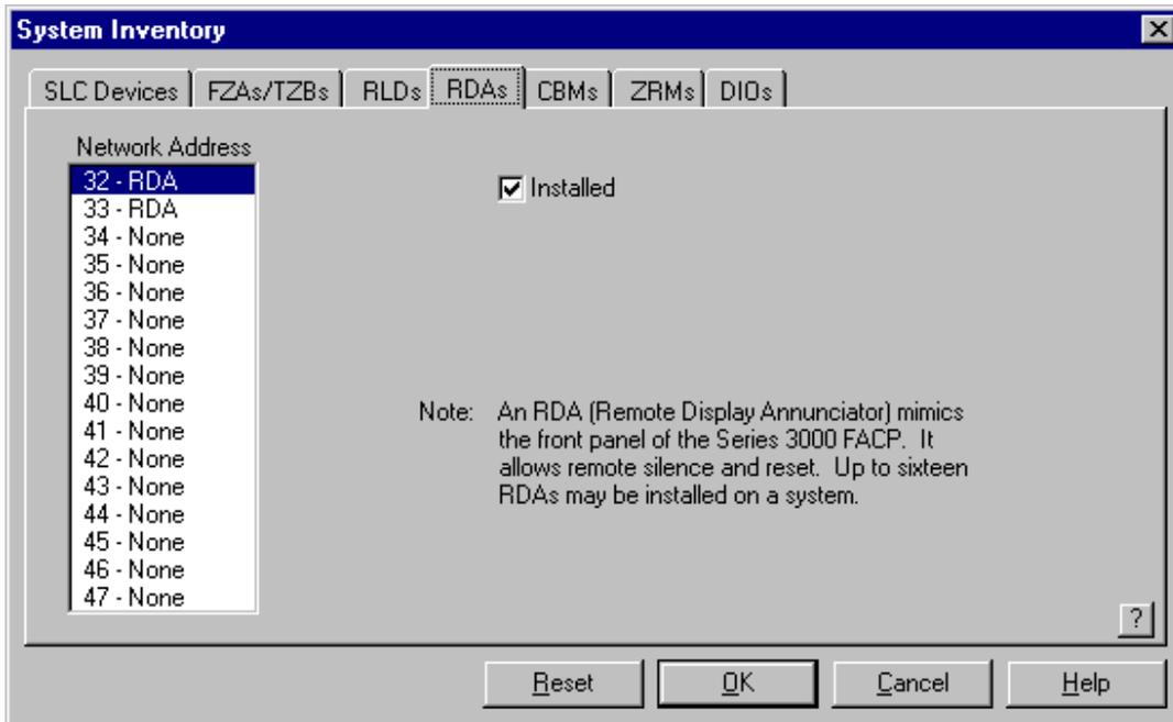
This page of the System Inventory dialog allows you to configure the number and addresses of remote LCD displays.
