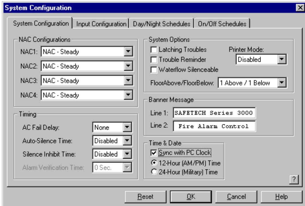
The "System Configuration" tab of the System Programming dialog is where general global system items are set. These include:
