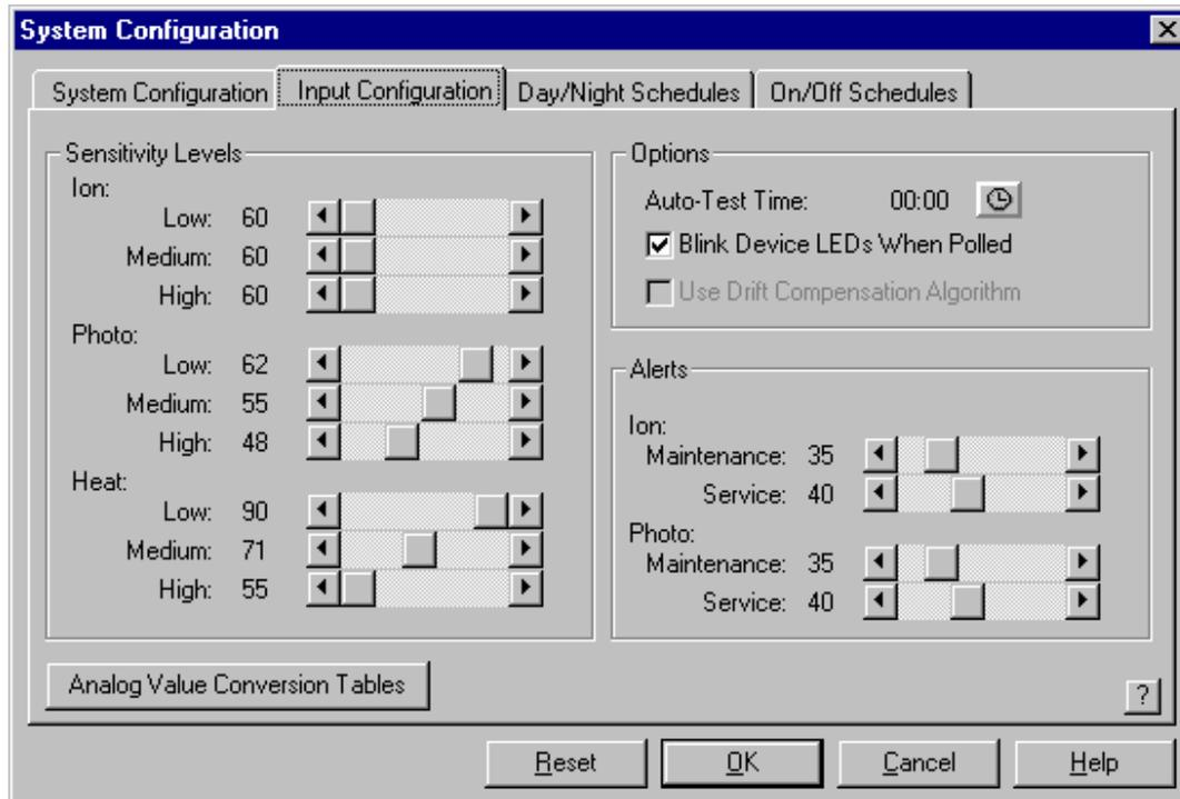
The "Input Configuration" tab of the System Programming dialog is where input sensitivities and options are set. These include:
