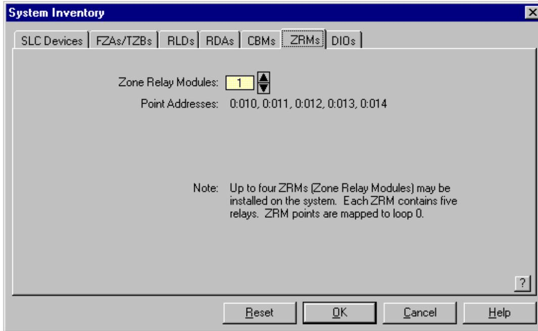
This page of the System Inventory dialog allows you to configure the number of relay modules installed. Up to four ZRMs (Zone Relay Modules) may be installed on the system. Each ZRM contains five relays. ZRM points are mapped to loop 0. Each relay can be assigned to any output group.
