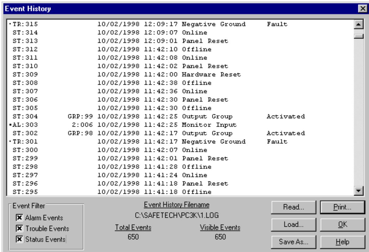
This dialog is used to view the panel's event history. Its main component is a large list box, which shows the events, one per line, newest to oldest. The first character of each line denotes its type: large dot = alarm, small dot = trouble, no dot = status). The remaining controls include:
