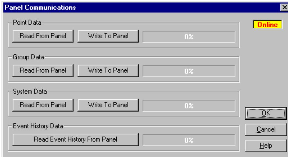
This dialog is used to transfer data to and from a Classic 2000 Mk II FACP. The "Online" indicator will show "Offline" if the panel is not connected, or if the program cannot communicate with the panel. Refer to the FAQ for help if you're having trouble getting the PC and the panel communicating.
