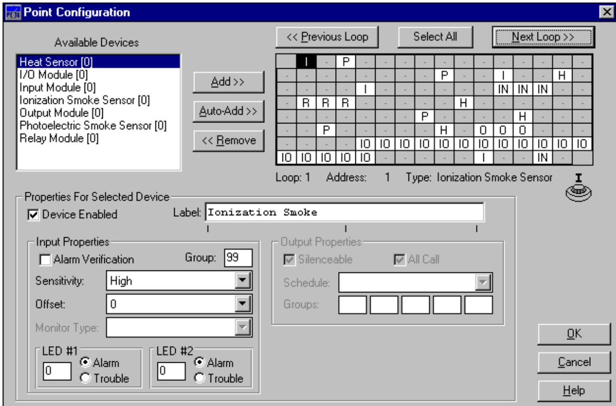
**NOTE: If Multiple Selection is going to be used to set alarm verification, sensitivity & output Group for a range of sensors, then the device label should not be entered until after multiple editing has finished, because multi-editing will also change the device label.**
