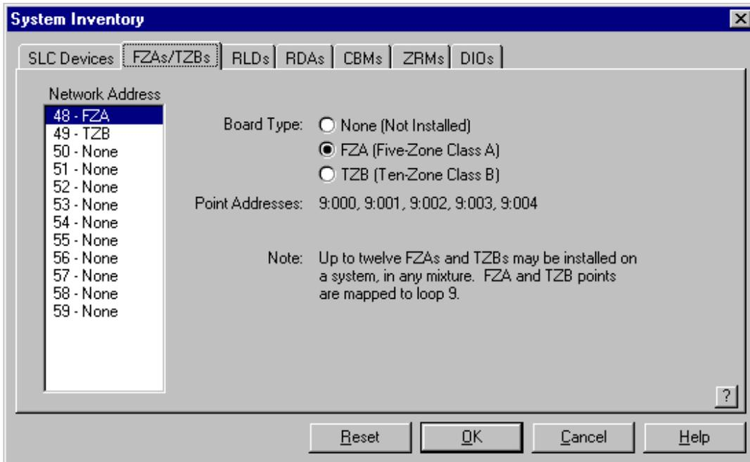
This page of the System Inventory dialog allows you to configure the number and addresses of conventional zone input cards installed on the RS-485 network.
