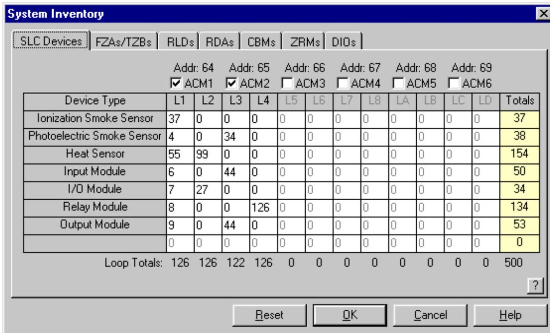
This page of the System Inventory dialog allows you to configure the types and quantities of SLC devices installed on loops 1-8 and A-D.
