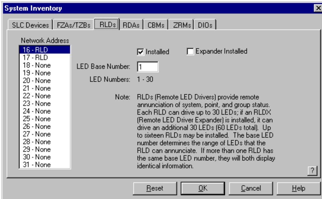
This page of the System Inventory dialog allows you to configure the number and addresses of remote LED display boards.
