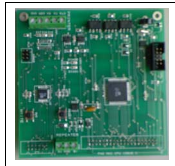
New CPU – 2 small surface mount ICs
