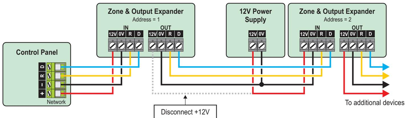
Remote keypads and expanders are all connected to the same network terminals located at the bottom left hand corner of the control panel and may be connected serially (daisy chain), in parallel (star) or any combination of the two.
